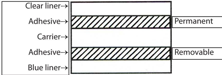
**Important:** Attach the side with the permanent adhesive to the graphic.
