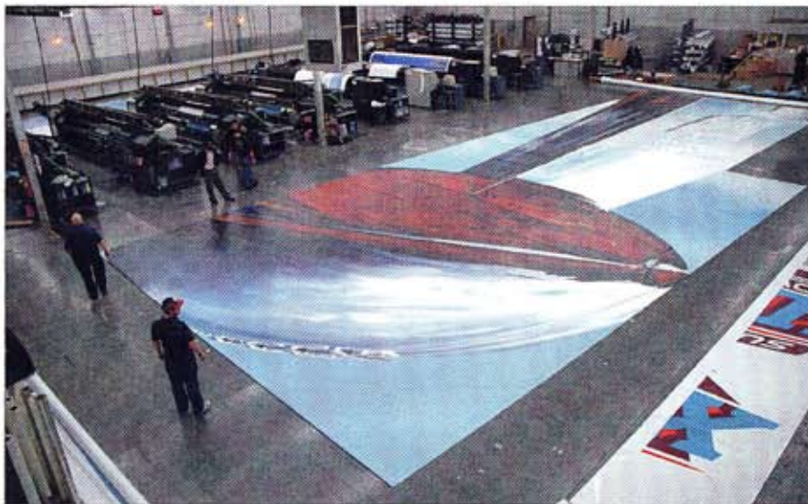
Vision International printed all graphics then RF welded them before shipping. This 81' x 32' graphic was printed on Mehler vinyl and installed in the south end zone.
