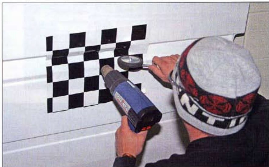
3M's Controltac IJ380 film can be used on extreme curves for concave and convex areas like this Dodge Sprinter door.
