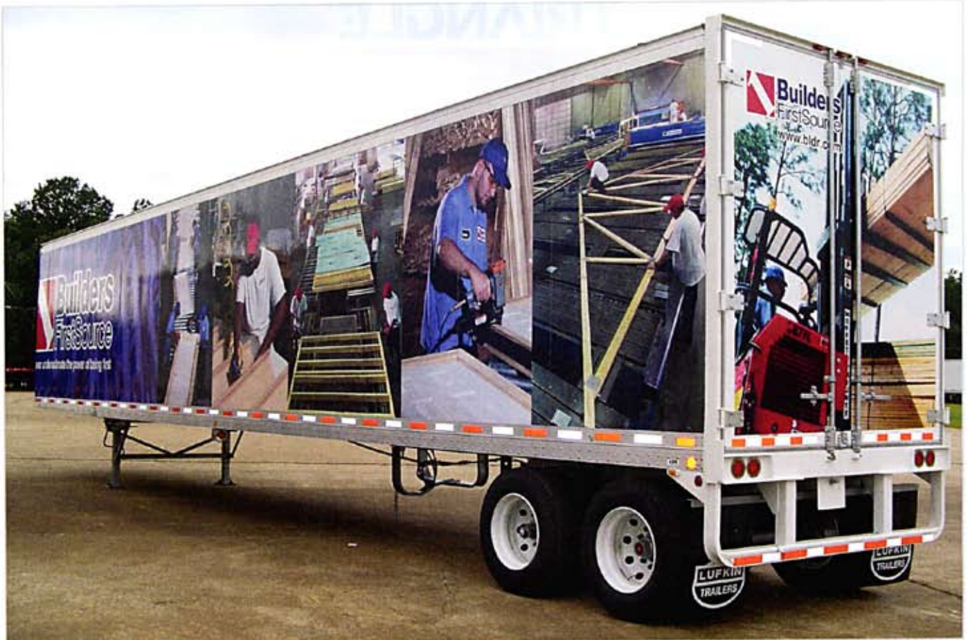
As part of a pilot program for Builders First Source, a select number of vehicles were made into marketing pieces. The vehicles were printed on the HP Scitex Turbojet using Avery MPI 1010 film for the digital portion of the project, while FT1002 and NV1500 cut vinyl were used for the logo, company name and text. The reflective portion is featured on the side of the trailer so it is more visible at night.
